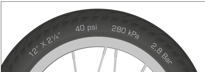
Illustr.: Tyre with tyre size specification (example)
